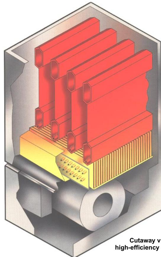
Cutaway view of a high-efficiency furnace
