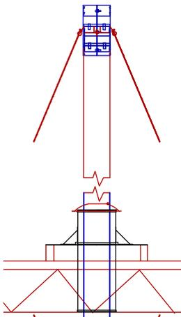
1. Install the Guy section 1 Vent section (2' length or less) below the Rain Cap Vertical Termination.
