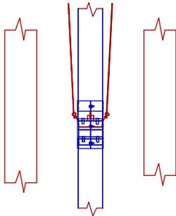
1. Install the (first) Guy section at approximately the mid point of any continuous vertical run but in no case further than 50 feet above or below a bottom support, roof jack or additional Guy Section. On single wall Saf-T Vent systems the Guy Section attaches exactly as described in the Saf-T Vent Installation and Maintenance Instructions. On double wall Saf-T CI Vent systems the Guy Section requires the special notched Coupler specially fitted around the anchor tabs.
